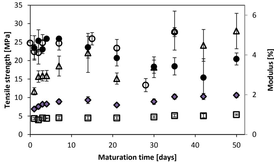
**Figure 4: Mechanical properties of films prepared from IR0401 latex compound with 5phr Bostex™862 as a function of maturation time.**
