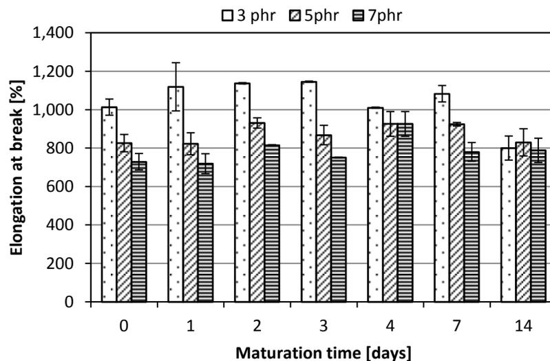
**Figure 2: Elongation at break vs. maturation time for IR0401 films cured with Bostex™851 at three concentrations – 3phr, 5phr and 7phr.**
