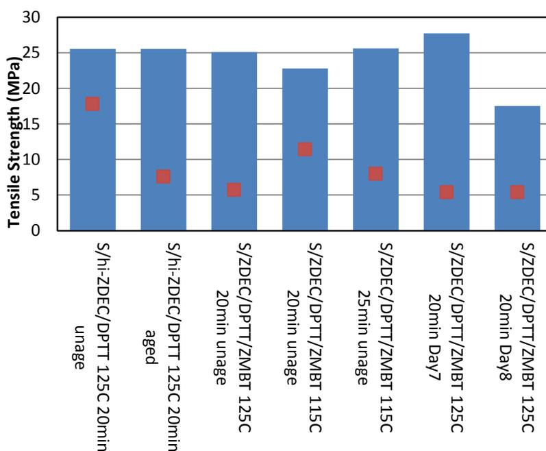
**Figure 10: Tensile strength of films made from compounds containing an added semi-ultra accelerator. The compounds were allowed to mature at high temperature of 28-33°C for 24 hours and then stored at 23-25°C. “hi-ZDEC” represents formulations containing ZDEC above 1phr. The red squares represent the coefficient of variance in the experimental data.**
