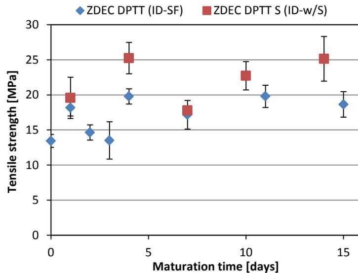
**Figure 9: Tensile strength vs. maturation time of films prepared from Cariflex® IR0401 compounded with (i) cure formulation free of elemental sulfur (ID-SF) and (ii) cure formulation with additional elemental sulfur (ID-S).**
