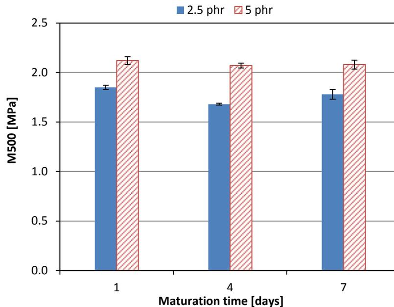
**Figure 15: M500 vs. maturation time of films prepared from Cariflex<sup>®</sup> 2GL compounded with Bostex<sup>™</sup>866 at two different concentrations (i) 2.5phr and (ii) 5phr**
