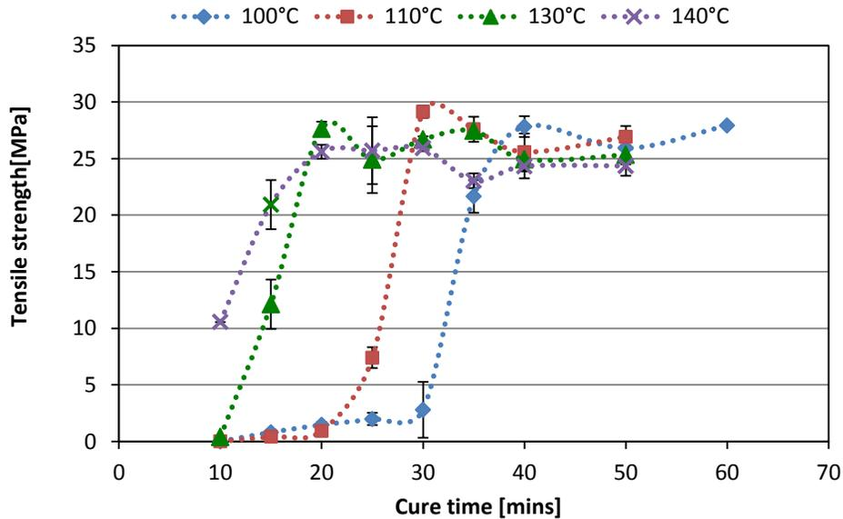
**Figure 3: Tensile strength vs. cure time for films prepared from IR0401 latex compound with 5phr Bostex™862 and cured at different temperatures.**
