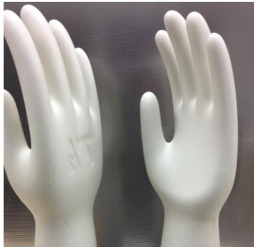
**Figure 11: Picture of cured film on glove former showing no blistering or bulging. IR0401 compound prepared with individual dispersions of cure chemicals, containing a semi-ultra accelerator was used for preparing the gloves. The compound was matured at a temperature of 28-33°C 24-48 hours prior to dipping.**
