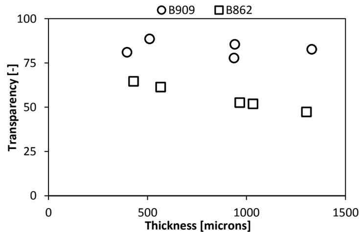
**Figure 7: Transparency vs. film thickness for films made from Cariflex® IR0401 latex compounded with Bostex™ 862 and Bostex909**
