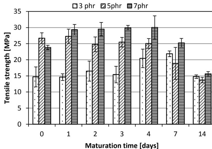
**Figure 1: Tensile strength vs. maturation time for IR0401 films cured with Bostex™851 at three concentrations - 3phr, 5phr and 7phr.**
