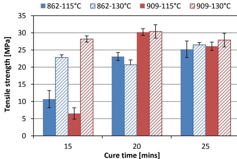
**Figure 5: Tensile strength of films prepared using IR0401 latex compounded with Bostex™909 and Bostex862 and cured for 15, 20 and 25 minutes at two different cure temperatures – 115°C and 130°C.**
