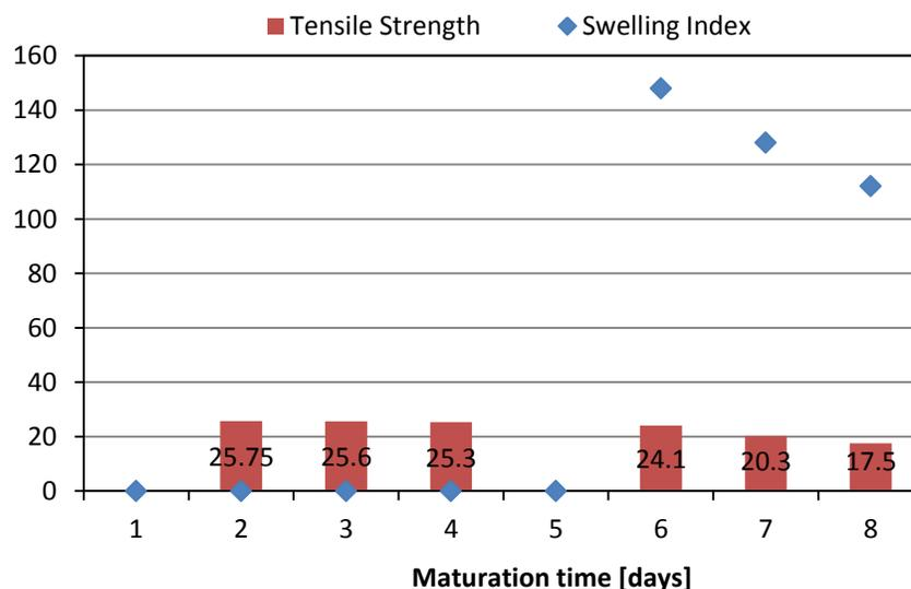
**Figure 12: Relationship of swelling index to deterioration in tensile strength as a function of compound maturation. (Swell index of 0 indicates that the film dissolved in toluene due to low crosslink density in the latex phase).**
