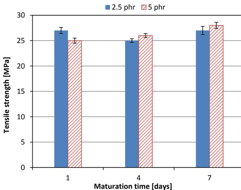
**Figure 14: Tensile strength vs. maturation time of films prepared from Cariflex® 2GL compounded with Bostex™866 at two different concentrations (i) 2.5phr and (ii) 5phr.**
