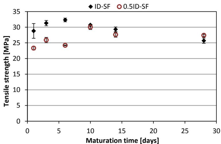
**Figure 13: Tensile strength vs. maturation time of films prepared using Cariflex<sup>®</sup> 2GL compounded with (i) ID-SF and (ii) 0.5ID-SF.**
