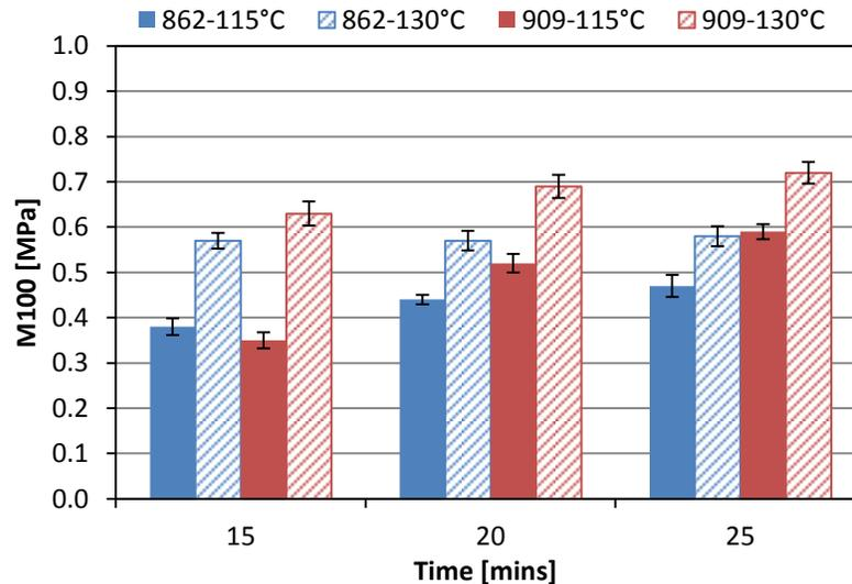
**Figure 6: M100 of films prepared using IR0401 latex compounded with Bostex<sup>TM</sup>909 and Bostex862 and cured for 15, 20 and 25 minutes at two different cure temperatures – 115°C and 130°C.**
