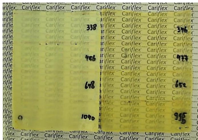
**Figure 8: Cariflex® IR0401 films of varying thickness prepared with (a) Bostex™ 862 cure package – appearance of film is opaque (film on the left) and (b) Bostex909 cure package – film appears much clearer (film on the right).**
